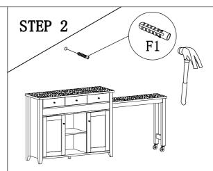
1. Use a light hammer to tap anchor into hole. 2. Anchor should fit snugly. If hole is too small, drill again to increase hole size. Do not force anchor into wall.
