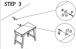
1. Insert drywall screw into metal bracket and into drywall anchor.
