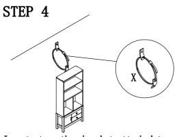
1. Insert strap thru bracket attached to wall. then thru bracket on item, and into head of strap. 2. pull lightly til strap stops. Assembly is complete.
