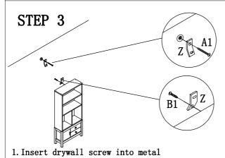
bracket and into drywall anchor.
