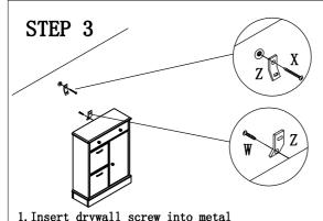
bracket and into drywall anchor.
