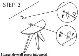
bracket and into drywall anchor.
