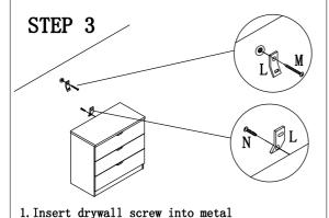
bracket and into drywall anchor.
