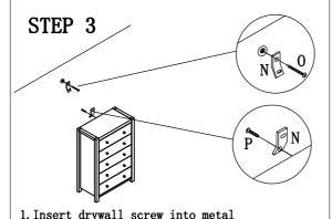
bracket and into drywall anchor.
