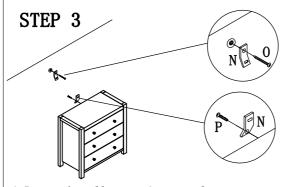
Insert drywall screw into metal bracket and into drywall anchor.
