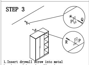
bracket and into drywall anchor.
