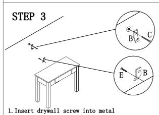
bracket and into drywall anchor.
