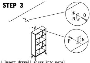
1. Insert drywall screw into metal bracket and into drywall anchor.
