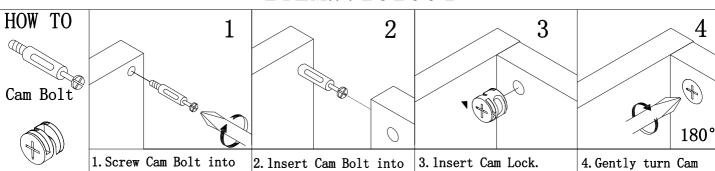
panel. bolt hole of joining Cam Lock pane1.
