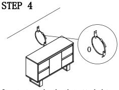
1. Insert strap thru bracket attached to wall. then thru bracket on item, and into head of strap. 2. pull lightly til strap stops.
