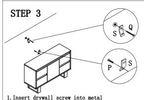
bracket and into drywall anchor.
